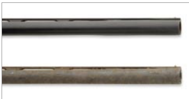
USING ACCELERATED SALT SPRAY TESTING, UNPROTECTED STEEL BARREL SECTION (BELOW) SHOWS CORROSIVE EFFECTS WHILE THE AQUA-TECHNOLOGY PROTECTED BARREL LOOKS BRAND NEW.
